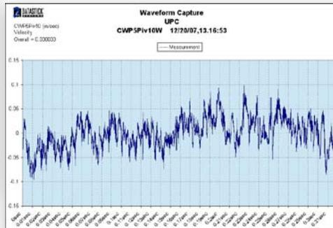
Velocity waveforms can transform either way: to acceleration or displacement waveforms.
