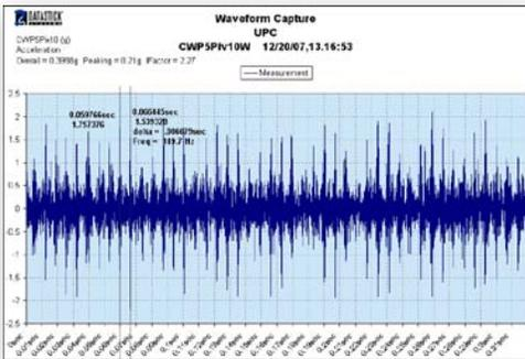
Here's the same bearing as above shown as an acceleration waveform. DAART lets you transform it into a velocity waveform, or a displacement waveform.
