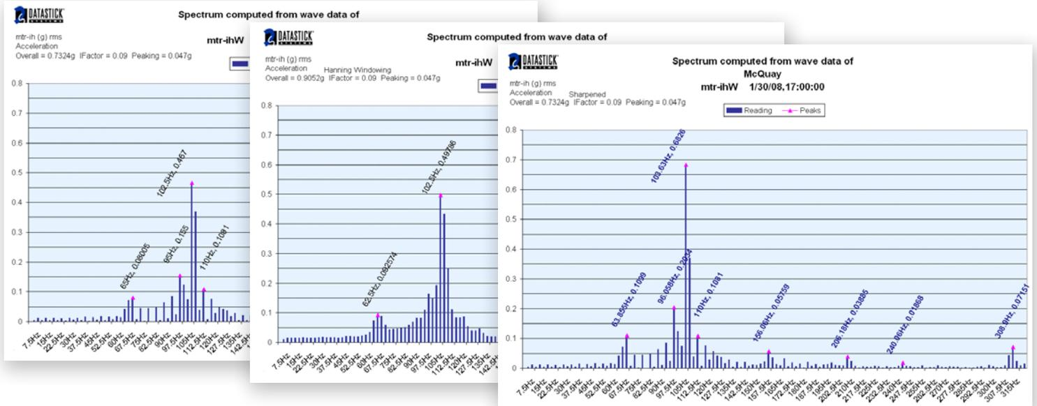
The FFT at left uses Rectangular windowing and shows several sidebands around an apparent 0.467 g peak at 102.5 Hz. The frequency display is limited by the 2.5 Hz FFT resolution chosen when the data was originally taken.
