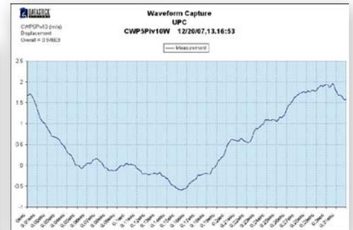
Suppose all you have is displacement data. You can create accurate velocity or acceleration waves with a single click.
