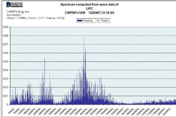
The haystack in this acceleration FFT shows you that *something* is going on with the bearing, but it doesn't tell you *what* is going on. You need demodulation to pull impact pulses out of the random noise so you can spot bearing faults early.
