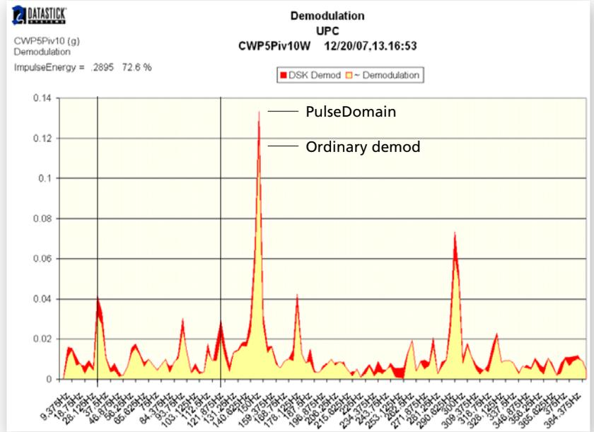
Datastick's exclusive PulseDomain demodulation's optimized signal to noise ratio can make the difference between seeing impact-pulse peaks easily and missing them. Using the same data as shown at left, here's the difference between ordinary demodulation (yellow) and PulseDomain demodulation (red). You might miss the importance of the peaks at 37.5 Hz and 118 Hz without PulseDomain.
